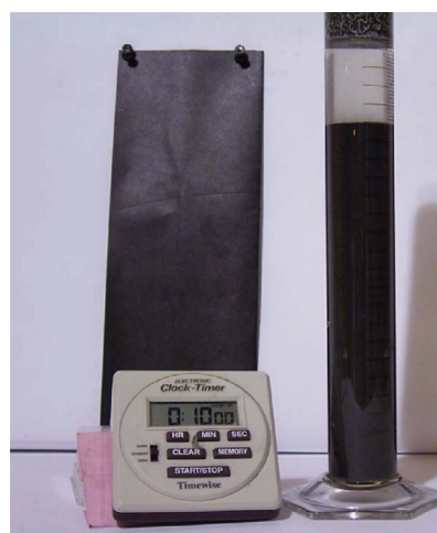
Figure 12—Stability measurement experimental set-up
